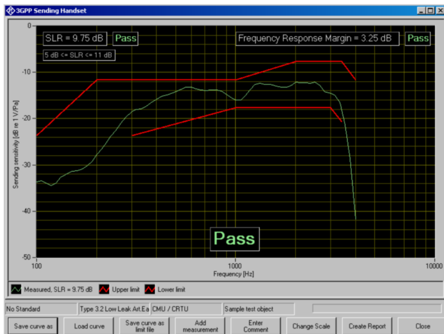
Fig. 18 Sending frequency response with SLR value displayed
