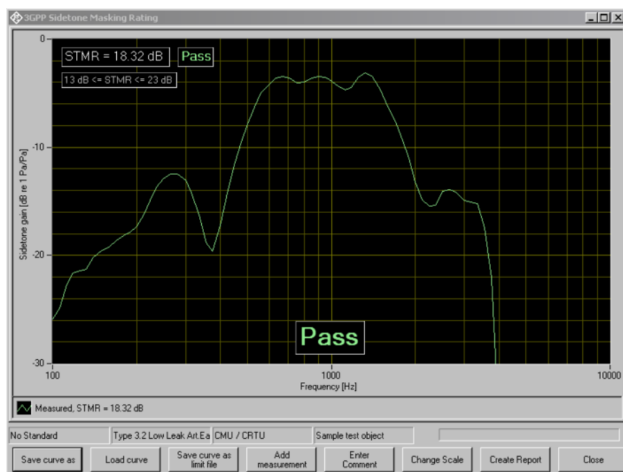
Fig. 20 Typical measurement of sidetone masking rating
